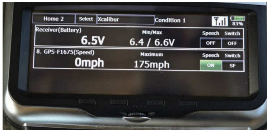
Photo of the 18MZ telemetry screen taken after a flight with the model stationary, but showing a maximum recorded airspeed of 175 mph
