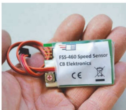
The unit is very compact and light, note the rotary switch, which is used during the set-up procedure
