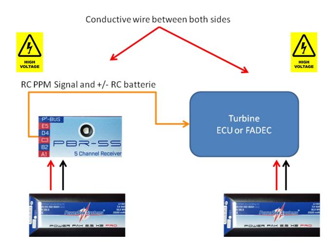
If you would make the same ohm meter measurement in the above installation with the conductive wire of the ECU that has no galvanic separation circuit, then you would get the following result.
