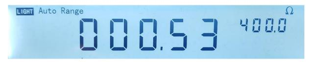
0.50hm, close to zero! This is more or less the conductive wire between ECU and receiver that you measure. By the way, everything less than 100K ohm is rated as conductive. This ECU has no galvanic separation. In case that an ESD would occur, this voltage pulse then can easily damage or destroy the sensitive 2.4Ghz chip set at the receiver side. In the installation with the galvanic separation this <u>can`t</u> happen.
