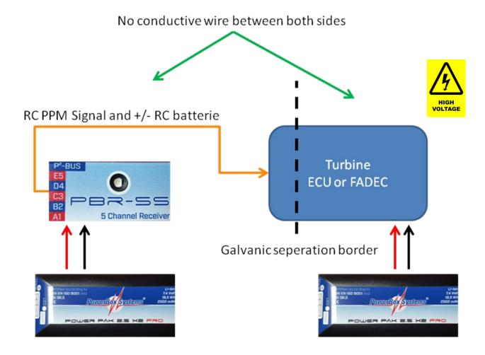
If you take an ohm meter and connect one lead of the instrument to the receiver minus GND pin and the other lead to the minus of the ECU/Fadec. If you measure high resistance in the range of some mega ohm. Please see ohm meter picture below as an example. Then your ECU has a galvanic separation.
