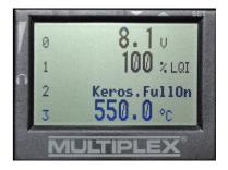
Supports the Multiplex Sensor Bus (MSB) with feedback of the current ECU measured values to Royal EVO, Profi TX or Cockpit M-Link Receivers. The MPX telemetry display (part number 45182) is supported as well.
